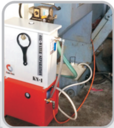
1 Place a suitable location Note the direction of the outlet.
