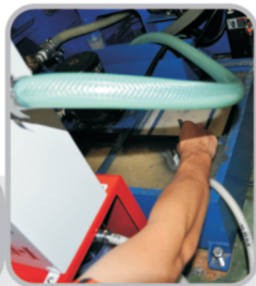
9 Measuring CNC water tank level,adjust the oil collect device height.
