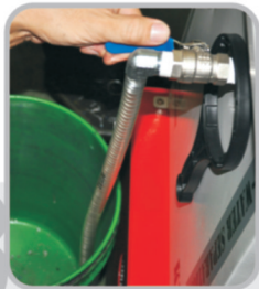
13 Look drain the oil window ,open the valve discharge of waste oil,using the bucket.
