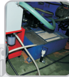
6 Put suction pipe into CNC tank and open intake valve for suction, into internal tank.
