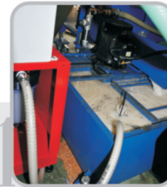
11 Adjusting oil collect device for suction level.
