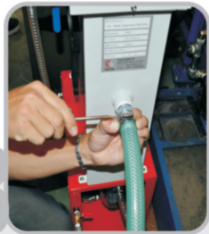
3 Use a screwdriver to outlet pipe connected to the discharge valve.
