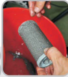
3 Cleaning filter cartridge by water or air gun.
