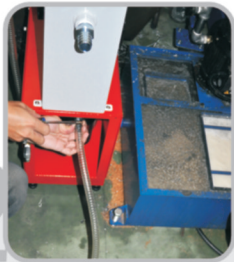
2 Use a screwdriver to 1/2 suction pipe connected to filter.
