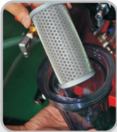
4 Put the cartridge into filter and check the filter O-ring.
