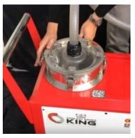
**5.** Insert the drain into the straight plug of the drain and lock it with a screwdriver.
