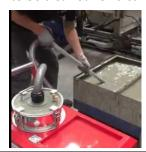
8. At the end, lift the suction pipe and close the pump actuation switch after the drain is no longer draining water.
